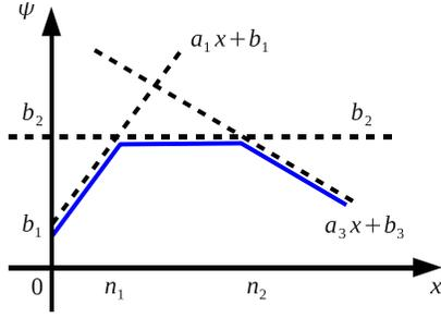
Figure 1. Example lower linear envelope  $\psi_c^H(\mathbf{y}_c)$  (shown solid) with three terms (dashed) as a function of  $x = \sum_{i \in \mathcal{C}} y_i$ . When  $x \leq n_1$  the first linear function is active, when  $n_1 < x \leq n_2$  the second linear function is active, otherwise the third linear function is active.
