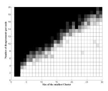
Figure 3. Simulation results for fully observed 1000-node graph with cluster of non-uniform sizes. The graph has clusters of at least size k. For different minimum cluster size  $K_{\min}$  and number of disgreement per node b, we plot the probability of success.
