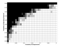
Figure 4. Simulation results for partially observed 400-node network with minimum cluster size fixed at  $K_{\min} = 60$ . Disagreements are placed on each (potential) edge with probability  $\tau$ , and each edge is observed with probability  $p_0$ . The figure shows the probability of success in recovering the ideal cluster under different  $\tau$  and  $p_0$ . Brighter colors show higher success.
